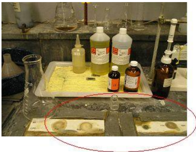
Figure 3 : Acid burns on the bench counter top.
