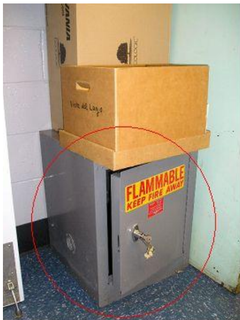
Figure 6: Flammable containment vault in the chemistry laboratory left open with combustible material stored on top.
