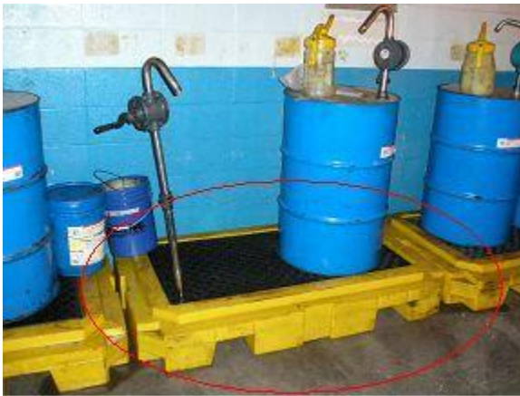
Figure 9: Secondary containment is adequate
