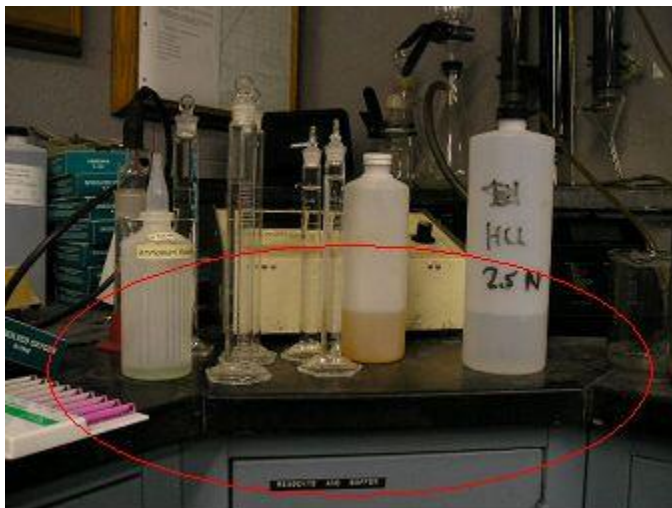
Figure 2: Acid and reagents left on the edge of the bench in the chemistry laboratory.
