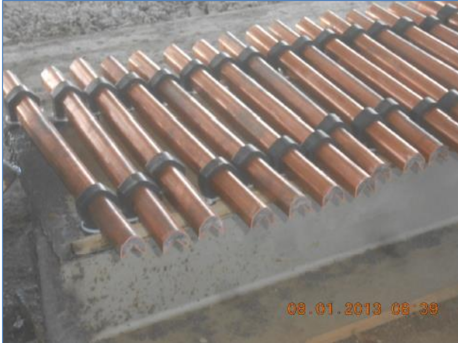
Photo 2: UNIGEL ® Linear Shaped Charges. Source: PG&E
