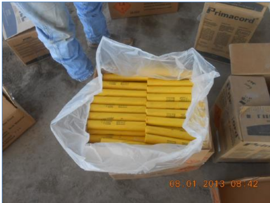
Photo 3: UNIGEL ® Kicker Charges. Source: PG&E
