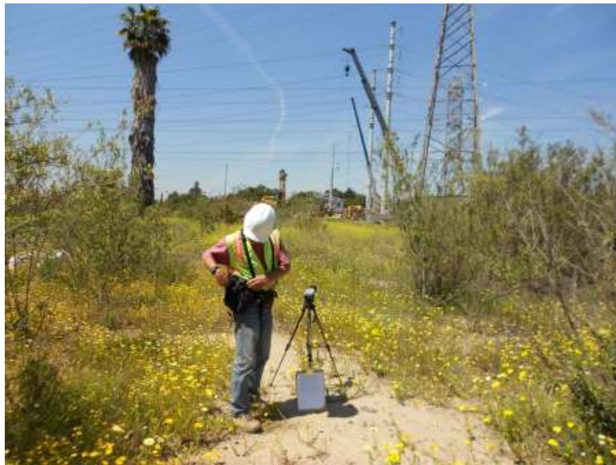
Figure 6: An ICF biologist checks a sound meter during work within a CAGN buffer at the San Gabriel Junction, Segment 8, Phase 4.
