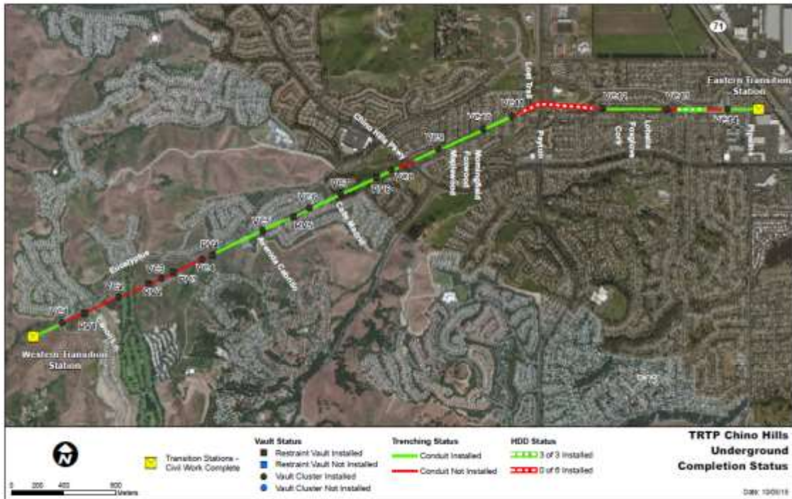
Exhibit A: 500 kV Underground Construction Status as of October 5, 2015.
