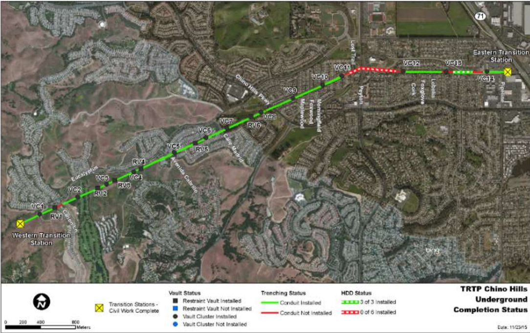
Exhibit A: 500 kV Underground Construction Status as of November 23, 2015.
