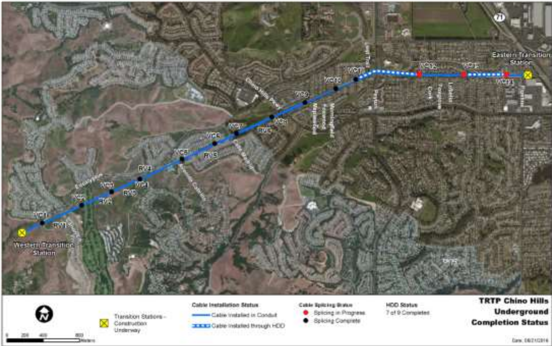
Exhibit C: 500 kV Underground Construction Status as of June 9, 2016.
