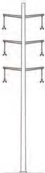
220-kV double-circuit TSP (Height Range: 70-200 feet)
