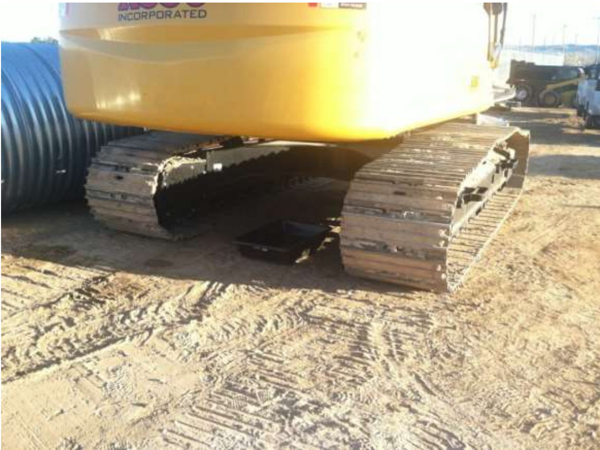
Figure 5 – Secondary containment is placed under machinery at the end of the day. View southeast, 02/26/15.
