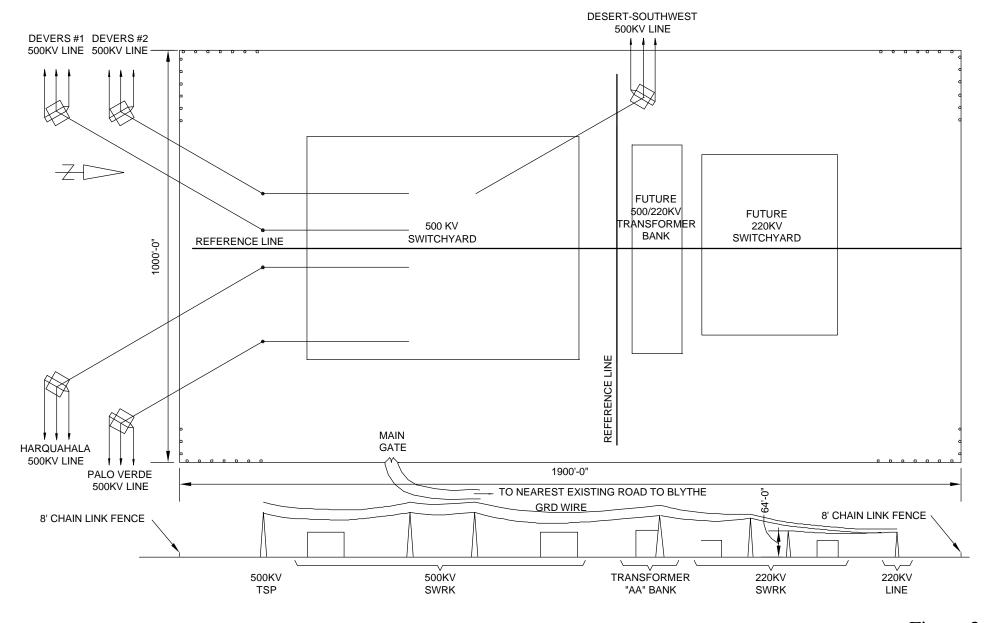
Figure 3-1 Midpoint Substation Block Diagram
