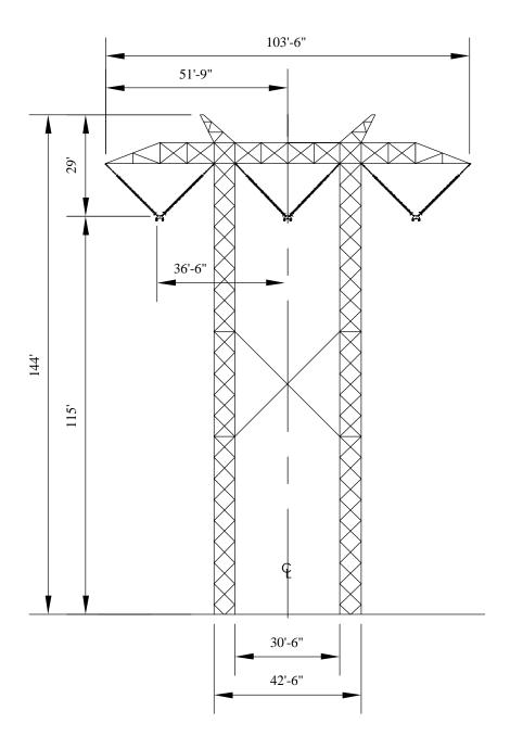
Figure 3-4 Typical 500kV Single-Circuit "H - Frame" Tower
