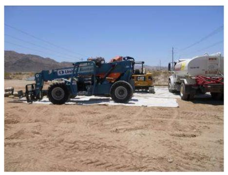
**Figure 9.** Inadequate secondary containment at the equipment parking area for the Series Capacitor site.
