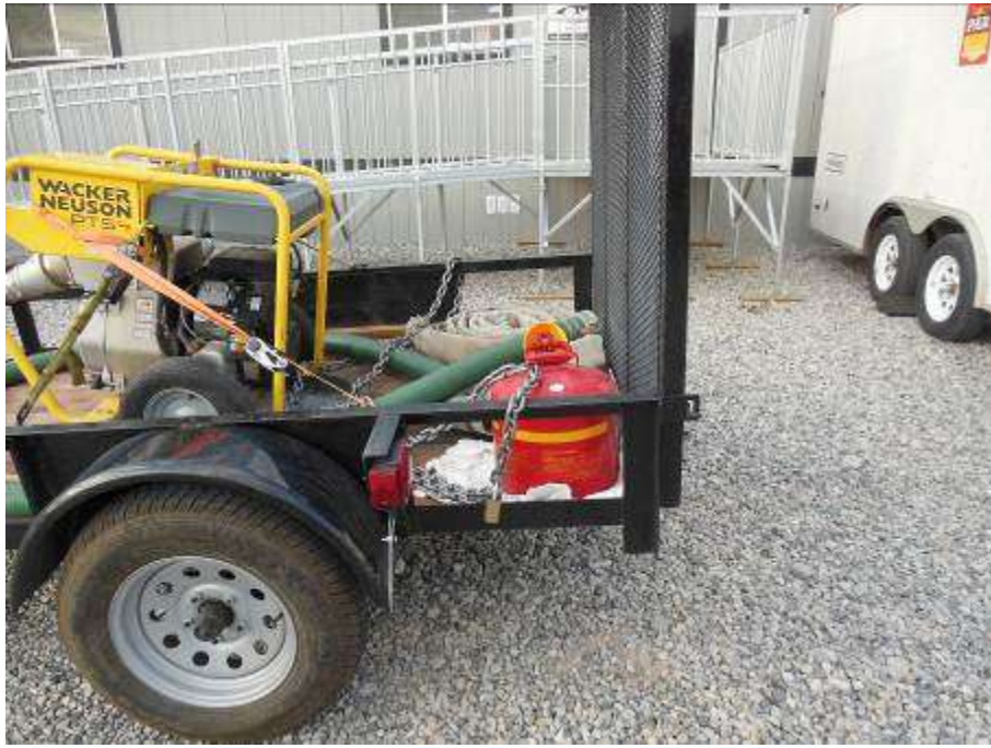
Figure 9. Gas can with no secondary containment at the Desert Center 1 Construction Yard.
