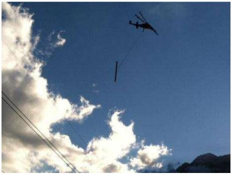
Figure 5. The KMAX helicopter flying an external load of bundled steel over the energized DPV1 Transmission Line.
