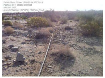
Figure 6. Equipment failure at Wire Site 31/Pull Site 32 (between Towers 2259 and 2260) caused one of the conductor wires to break free coming into contact with the ground. (Photo courtesy of FRED).
