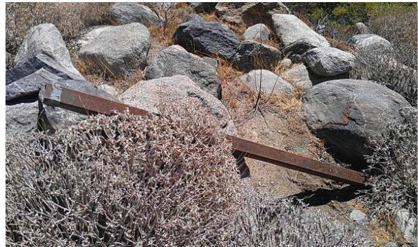
Figure 8. Micropile drill deck platform leg that dislodged and fell from the helicopter (Photo courtesy of FRED).
