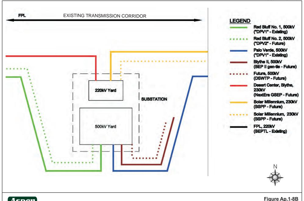
**Southern Alternative Substation Configuration (Perpendicular Orientation)**
