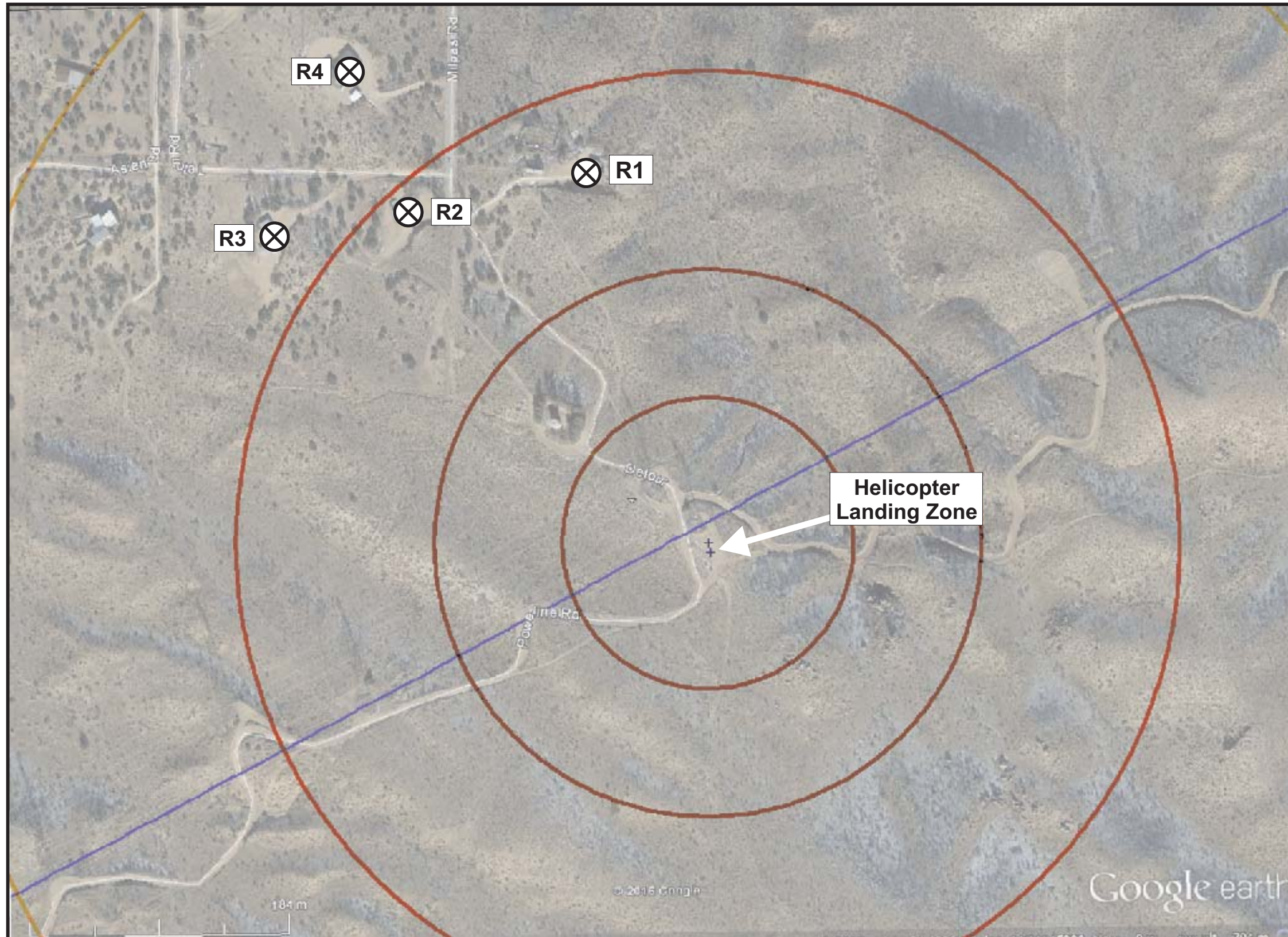
Satellite Aerial Photograph Showing Construction Equipment Noise Contours and Receiver Locations for Helicopter Landing Zone at Tower M16-T4 with 50% Helicopter Duty Cycle Job # B60102N1
