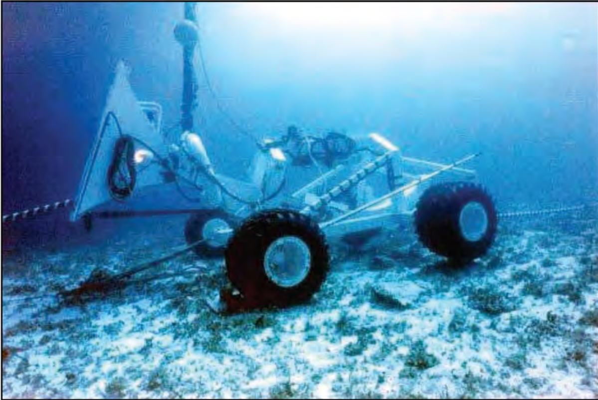
Actual hydroplow used in Trans Bay Cable project.
