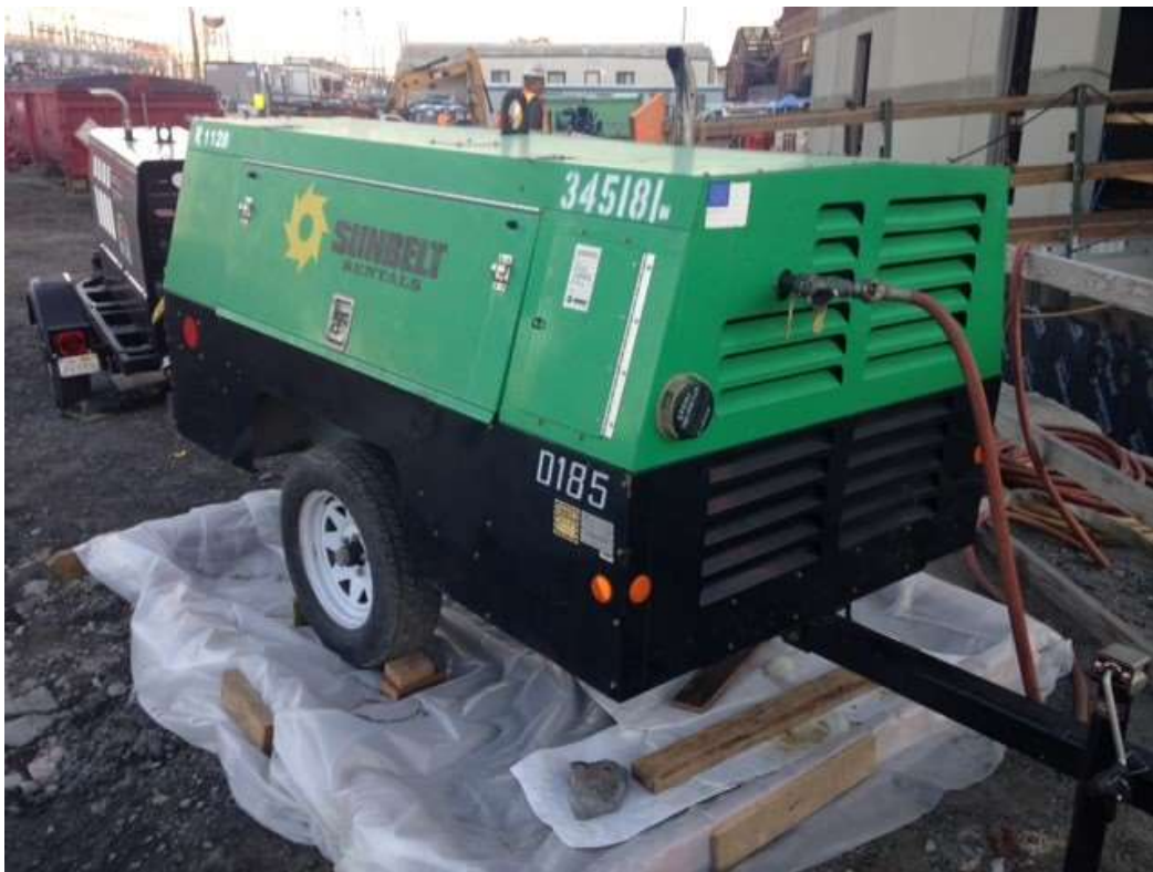
Figure 4 – Air compressor leaking antifreeze onto secondary containment. February 8, 2016. Photo courtesy of PG&E.
