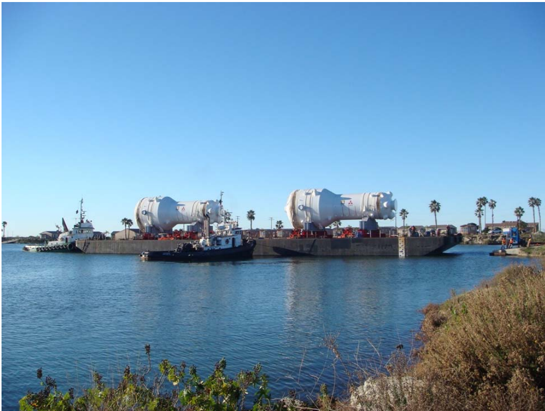
Figure 3: RSG barge arrival at the Del Mar Boat Basin at MCBCP. The RSG offloading was conducted over four days.
