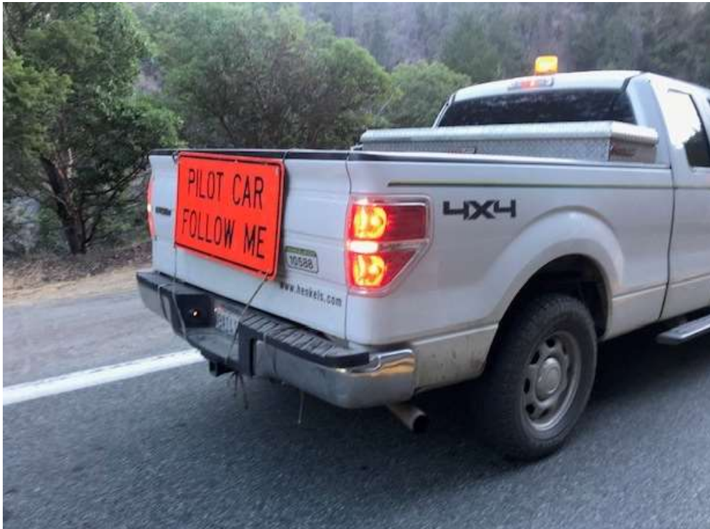
Figure 3 – Traffic controls and Pilot Car directing traffic through the construction site, September 11, 2019.
