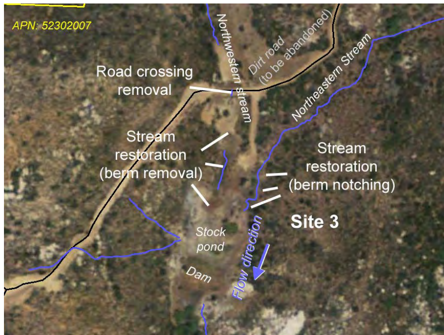
Figure 28. View of the large stock pond (reservoir), dam, road crossing, and northwestern and northeastern stream channels at Site 3 (aerial photograph taken 25 May 2009, source: Google Earth, accessed 2010). Present day road alignment shown in black and streams shown in blue.
