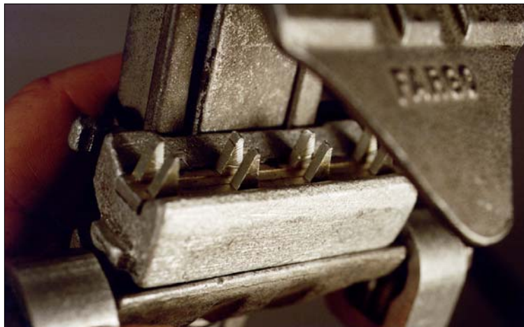
Figure 3-37 Piercing Hot Tap Clamp - Detail
