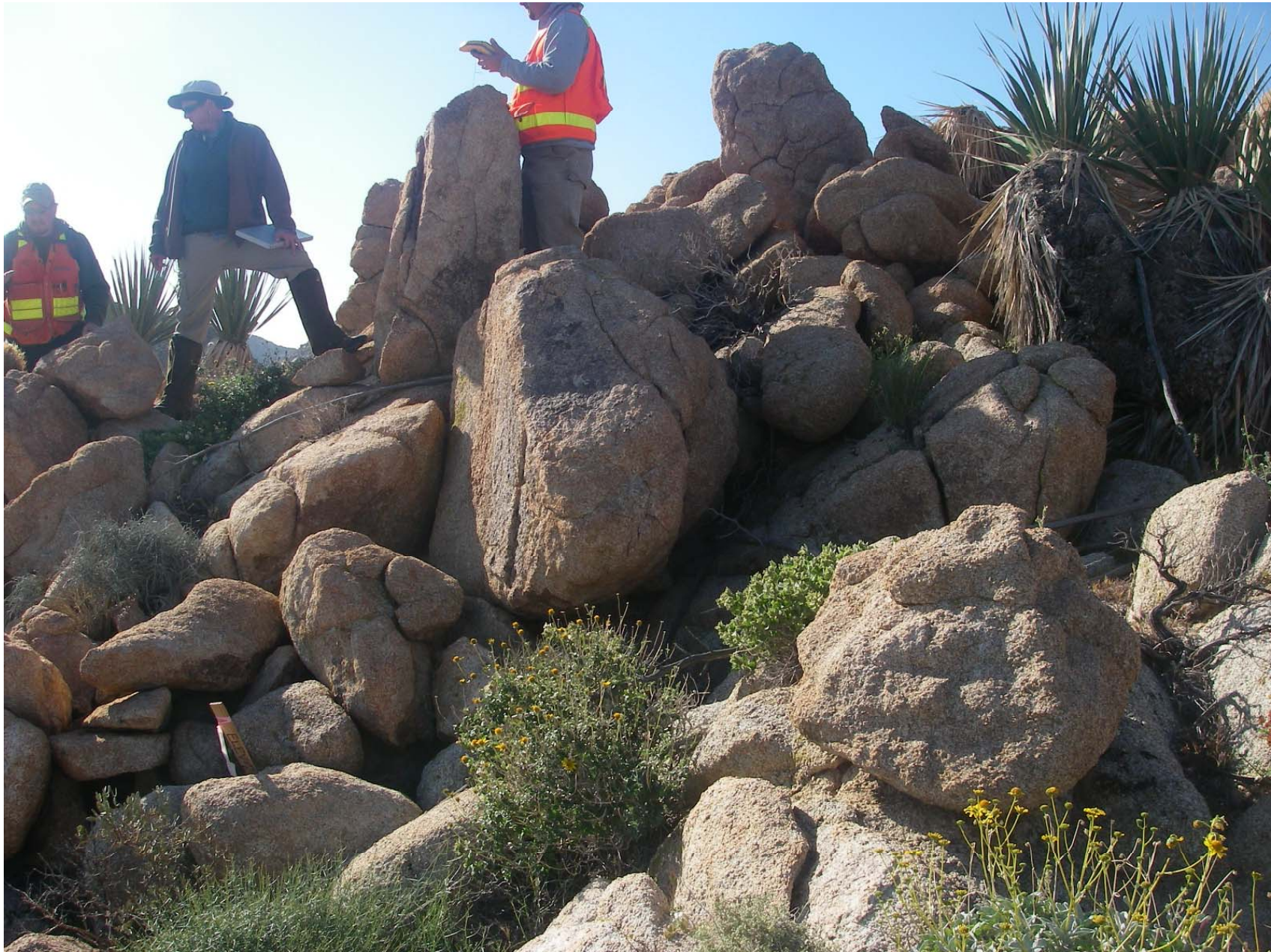
Tower 267-2: Rock fall hazard at Leg D
