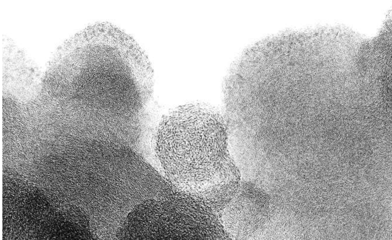
High Resolution Transmission Electron Micrograph of Carbon Black prior to graphitization
