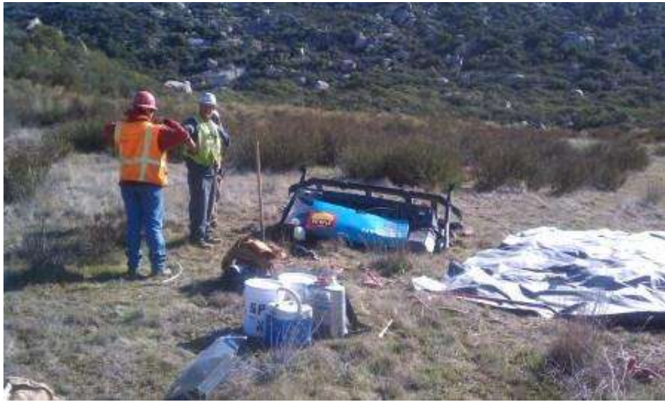
Figure 7: Air compressor destroyed after falling from a helicopter into a field. Crew is staging cleanup efforts. (Link 2)
