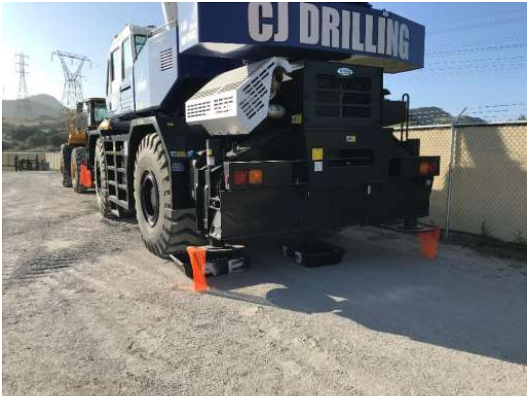
Photo 4 – Proper secondary containment observed at Poultry MY (April 5, 2018).
