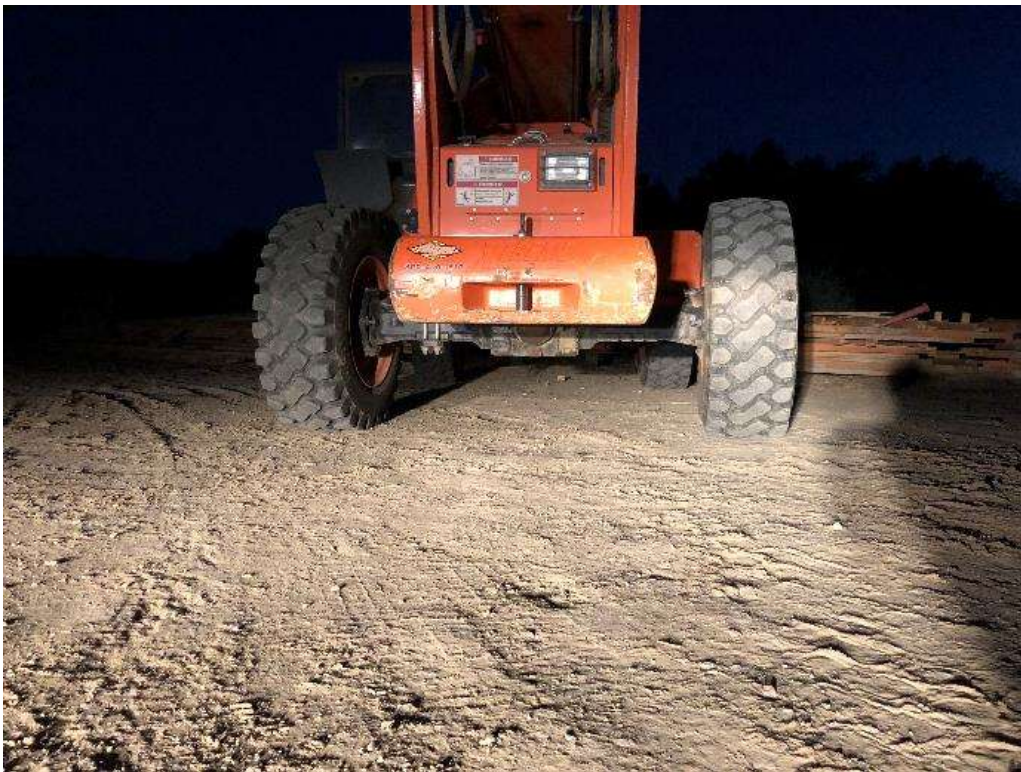
Photo 8 – Forklift staged overnight at Site 4N64 (Segment 4) without proper secondary containment (October 17, 2018).
