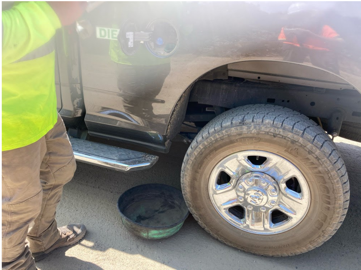
Photo 5: A drip pan was used during truck refueling along C 79B to prevent leaks and spills from being discharged into the soil in accordance with MM PHS-2 and the SRNP.
