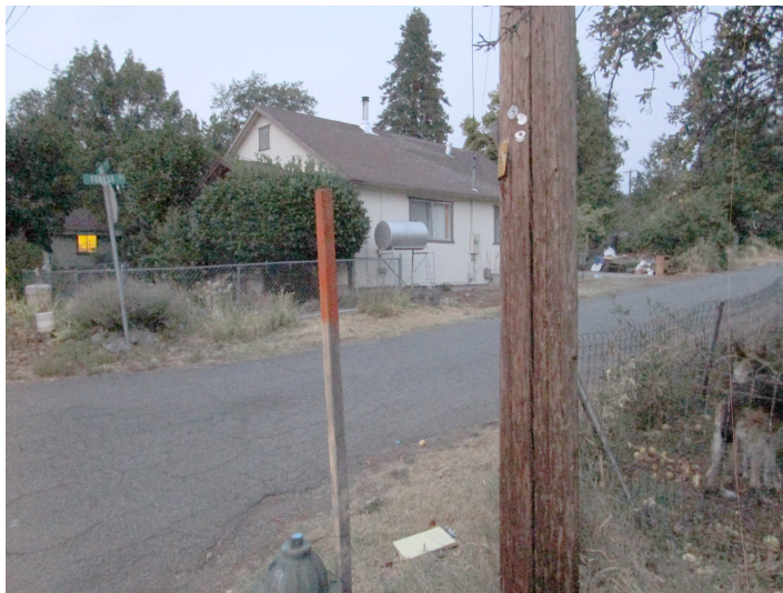
House at 412 Mill Street is 44 feet from Project's power pole #167241 as determined with laser distance measurer
