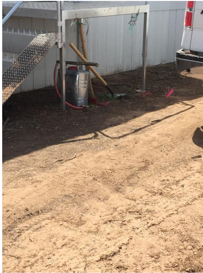
Photo 4: Fire prevention tools (including a shovel, Pulaski, and 5-gallon water pack) were staged on site and in vehicles in accordance with MM HAZ-4.
