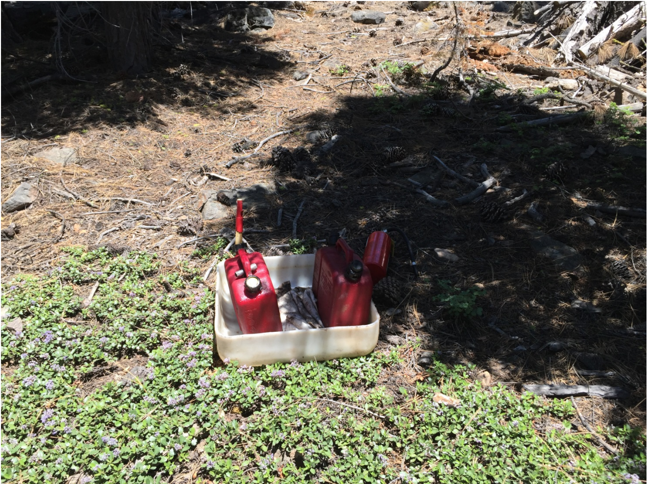
Photo 1: Chainsaw fuel kept in secondary containment (APM-WQ-1).
