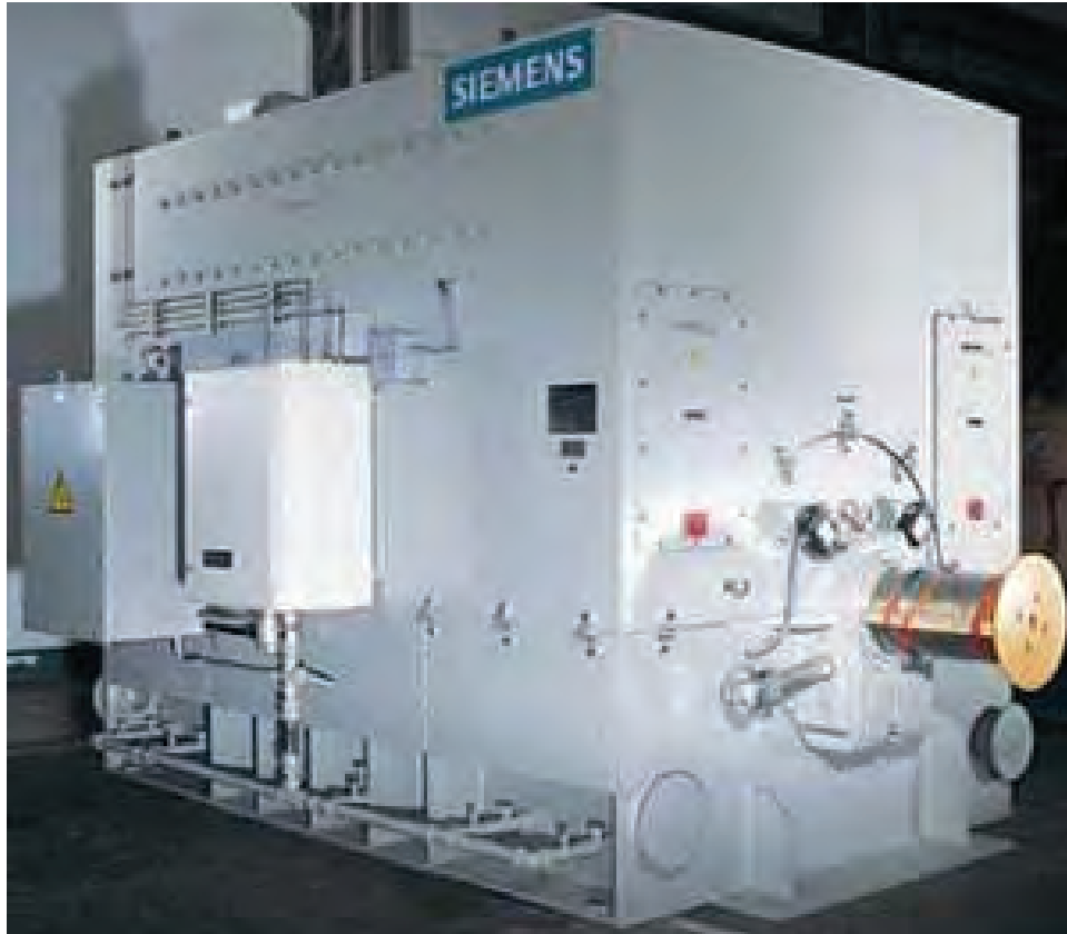
Figure 7 – Typical Synchronous Motor
