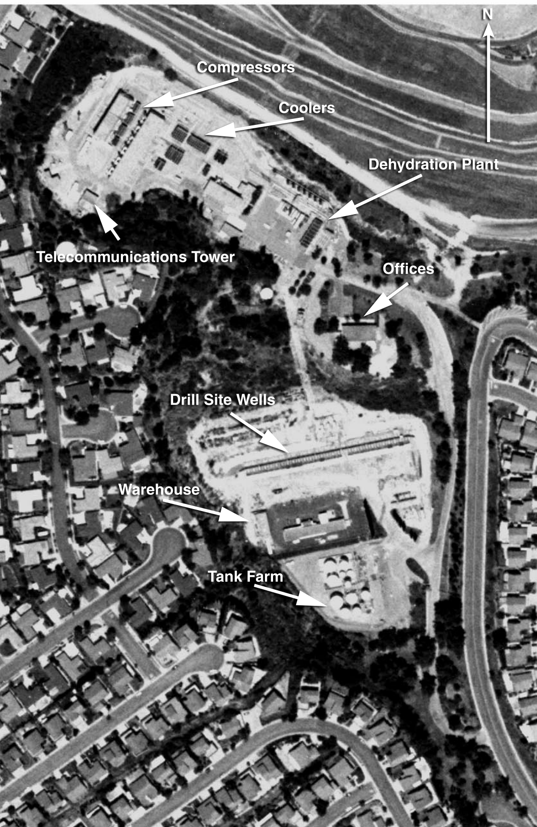
Figure 2.2-2: Annotated Site Map of Main Facility
