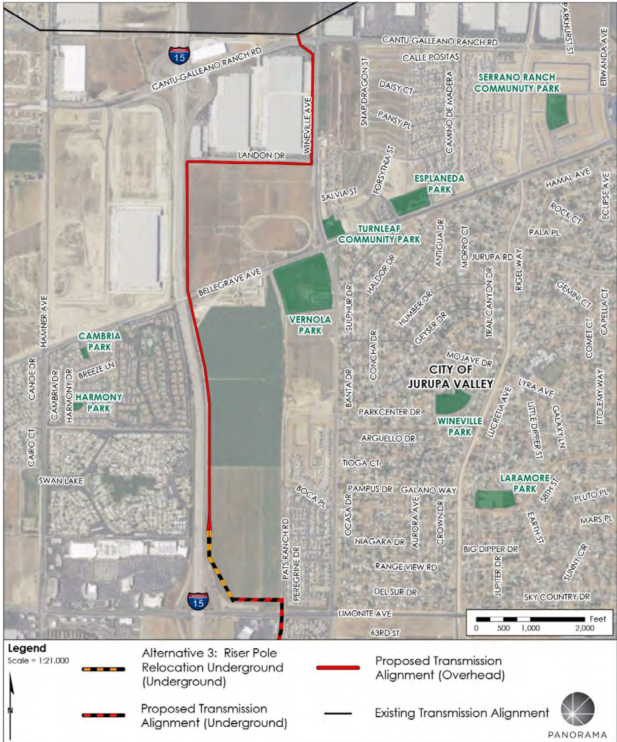
Figure 4.2-3 Alternative 3: Relocate Northern Riser Poles
