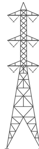
Lattice Steel Tower
