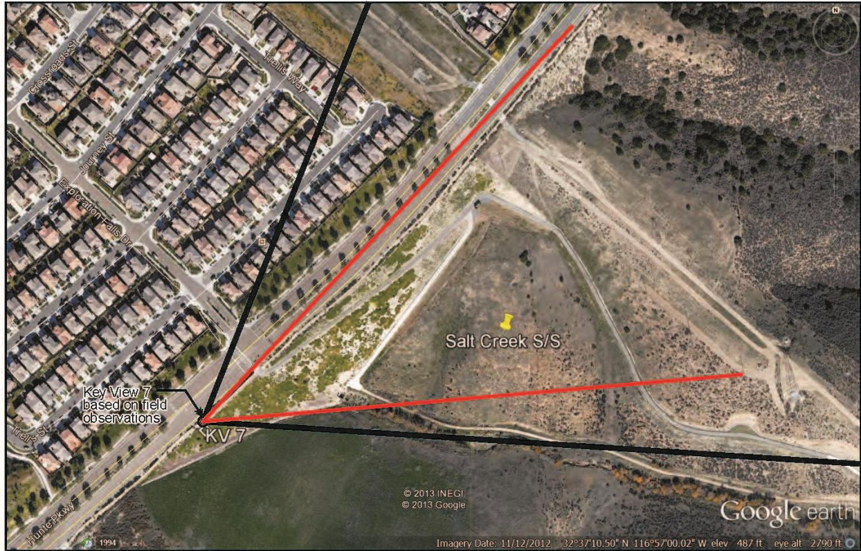
Exhibit 1 - This graphic shows the locations of the GPS supplied coordinates for Key View 7 and the location of the view from investigations on the site visit. The 2 black lines are the horizontal field of view shown in the SDG&E supplied baseline conditions and the visual simulations. The 2 red lines are the industry standard 40° view cone which would be captured using a 50mm focal length equivalent camera lens. Exhibits 2 and 3 graphically demonstrate the dichotomy that exists between the 2 approaches.
