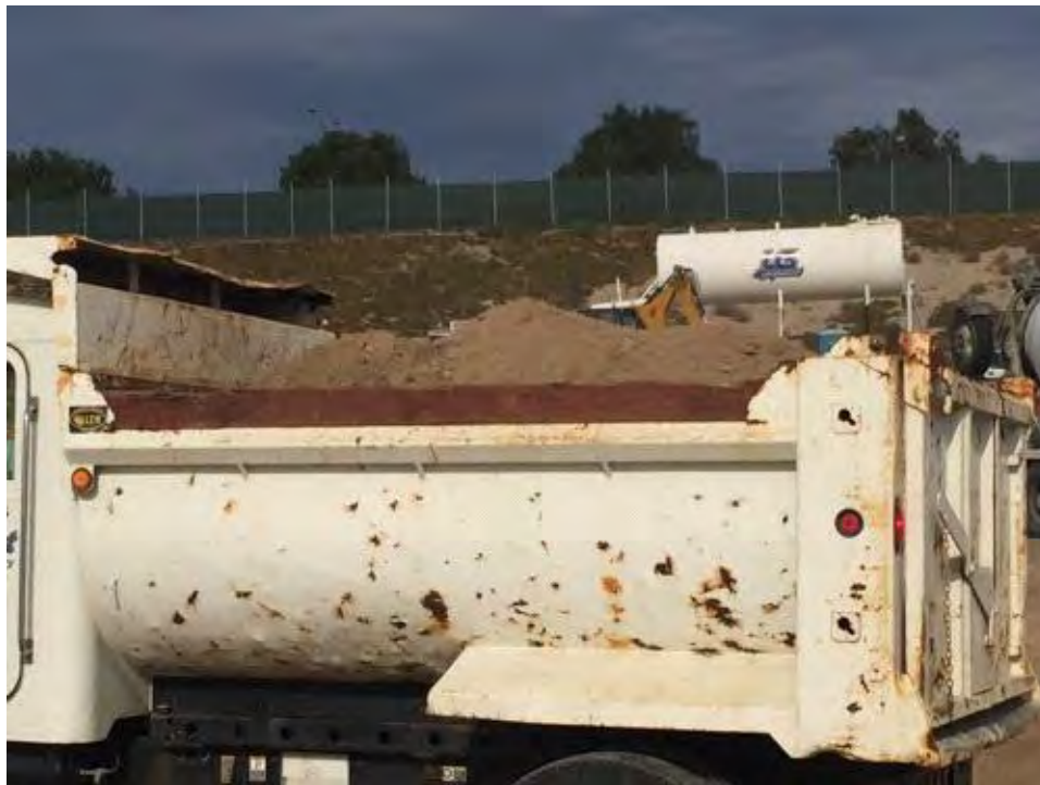
Caption Truck overloaded. APM AIR-1 requires load covering or at least 2 feet of freeboard.
