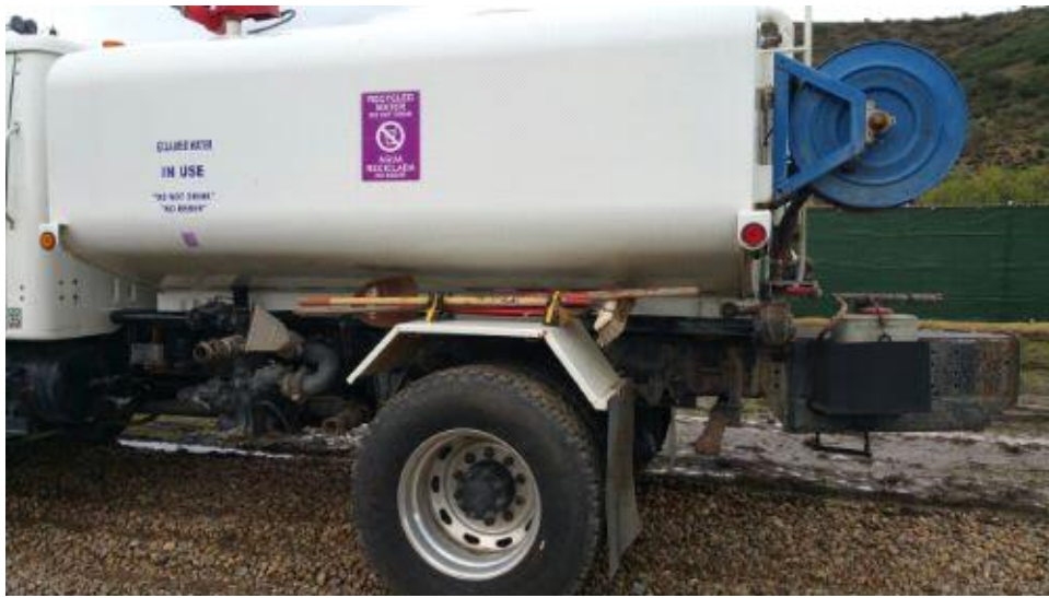
Caption Recycled water truck with appropriate signage and fire suppression equipment. Stonebridge.
