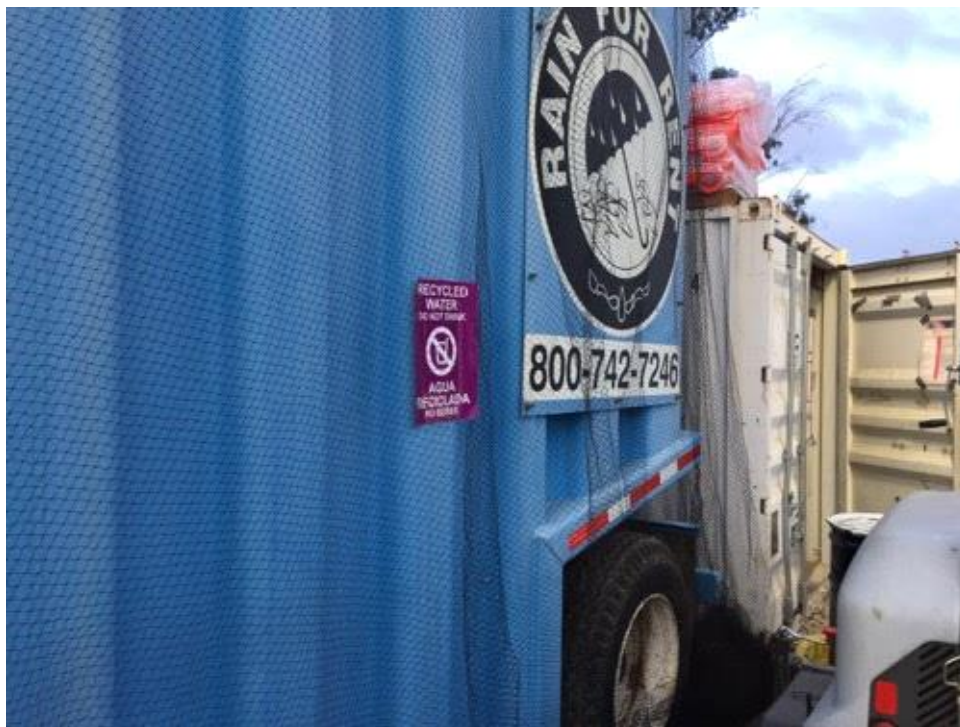
Caption Bird netting on water tank.
