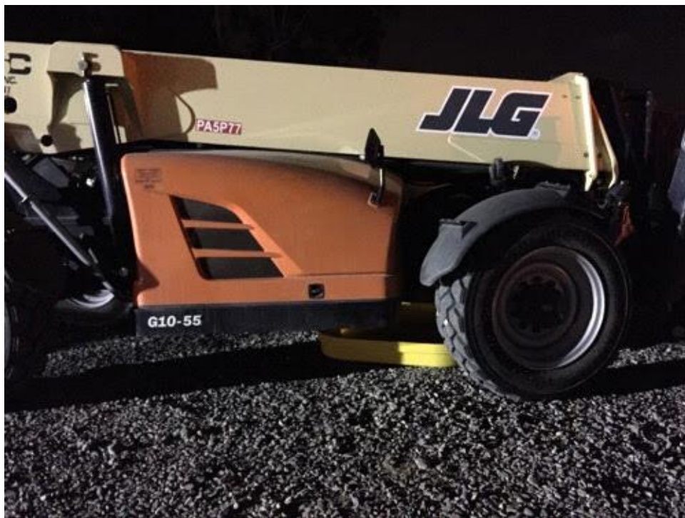
Caption Drip pans in place in storage yard.
