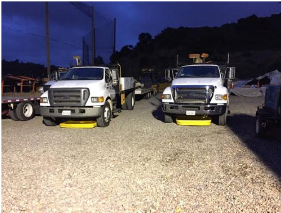
Caption Drip pans in place as required.
