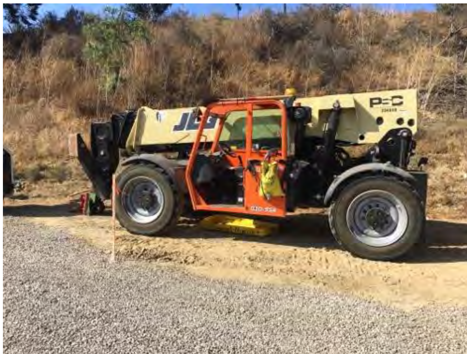
Caption Drip pans properly places beneath equipment.
