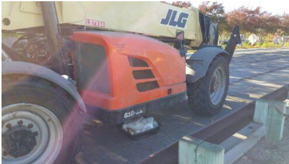
Caption Proper placement of drip pan on Stonebridge Parkway.
