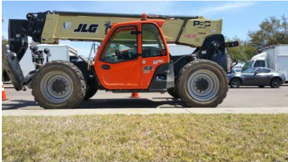
Caption No drip pan beneath SC4B34 at Padgett Road staging area.
