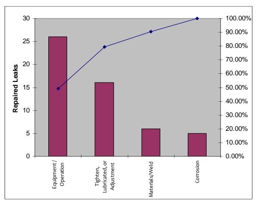
Figure 1 - Leaks by Cause
