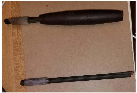
Figure 12: Fargo GL-115 Connector and Conductor
