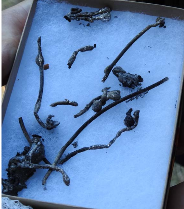
Figure 11. Failed pieces of conductor strands and evidence of arcing.
