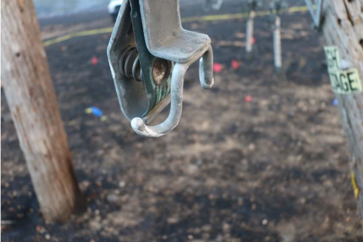
Figure 9. More signs of arcing (greenish coloring) on the fuses (Source: CAL FIRE)
