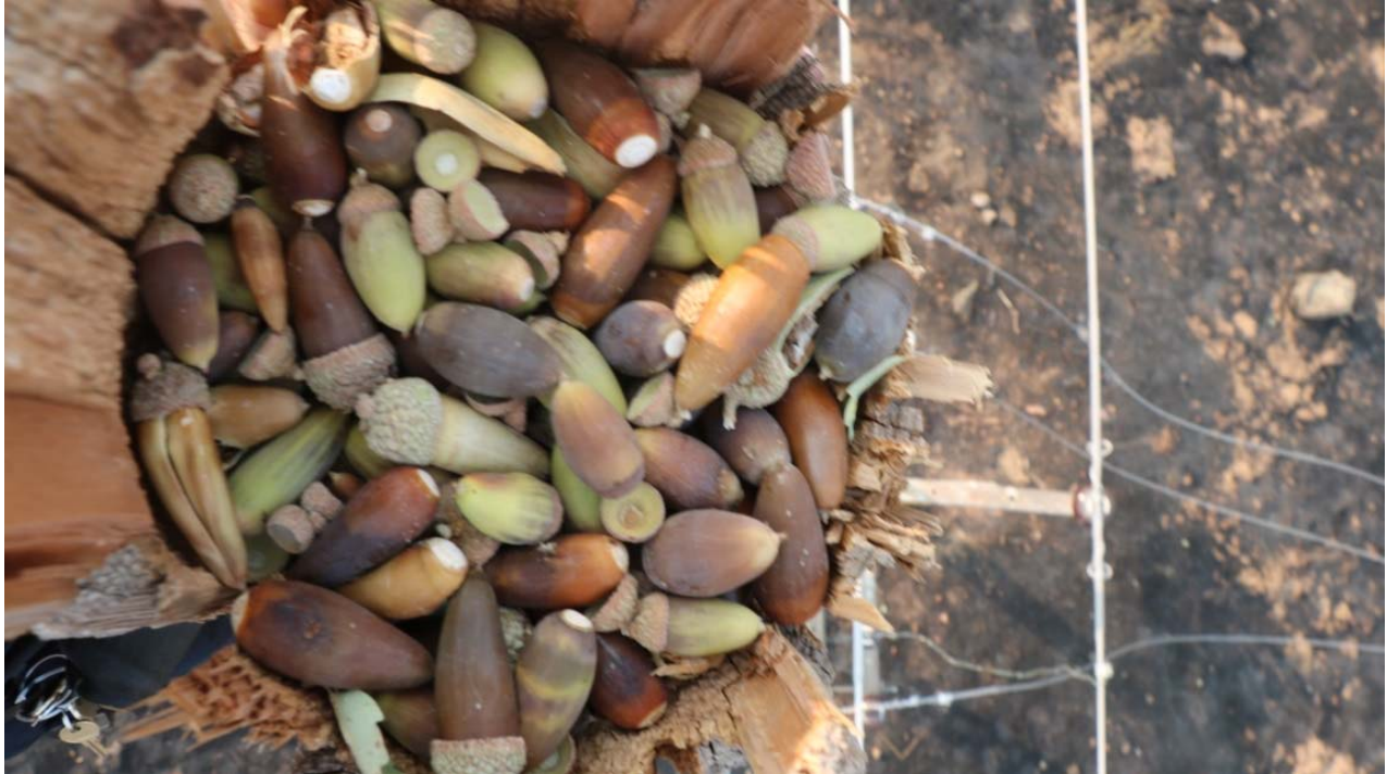
Figure 10. Top view of break on Fuse Cutout Pole 1447 full of acorns (Source CAL FIRE)
