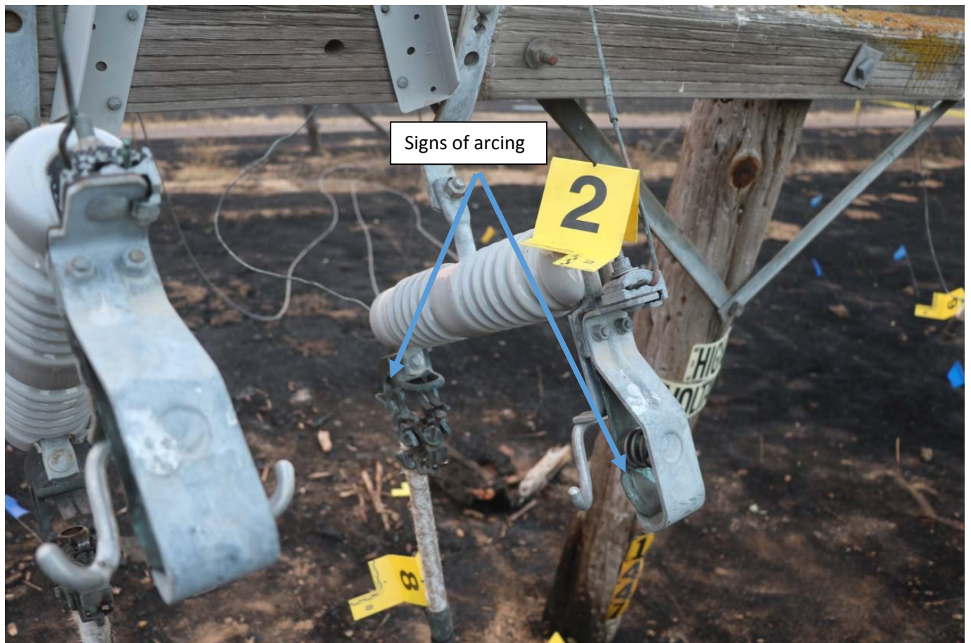
Figure 8. Signs of arcing on the fuses (Source: CAL FIRE)
