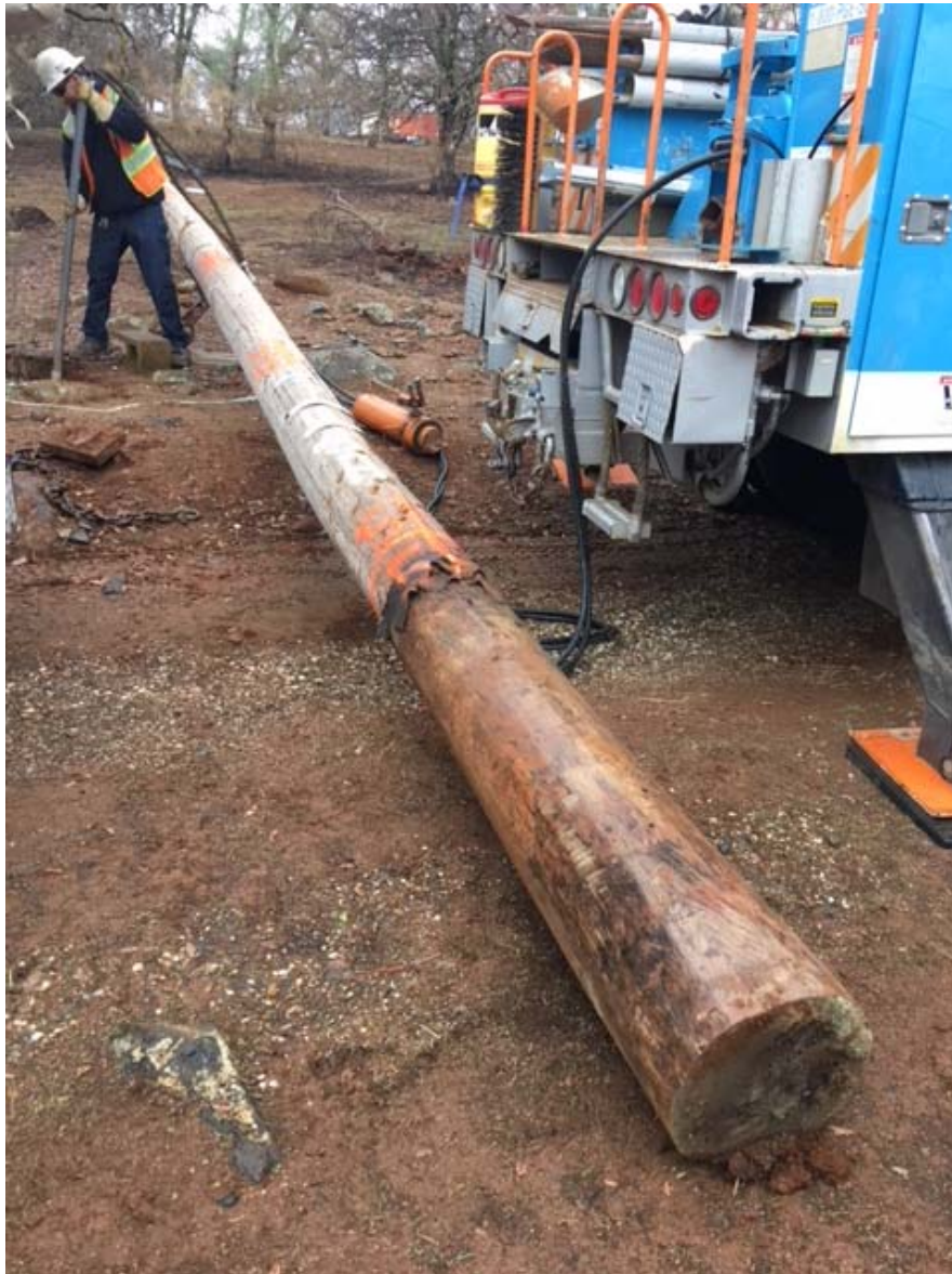
Figure 5. The subject 40-foot, Class 4 wooden pole.
