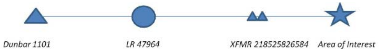
Figure 5. Diagram showing a transformer (denoted by XFMR) and protective devices upstream of incident span/Area of Interest. Not drawn to scale. (Source: PG&E 22 )
