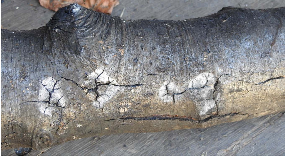
Figure 10. Metallic transfer on Alder tree limb. CAL FIRE evidence item number E-3.
